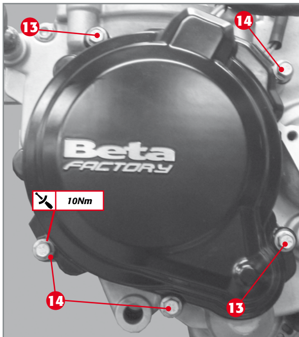
Flywheel cover coupled to crankcase.
