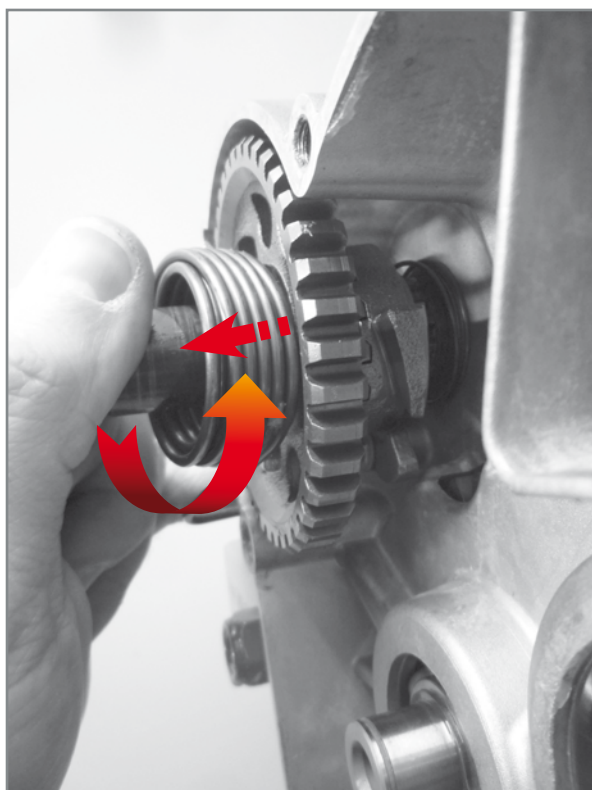
Extraction of shaft from crankcase.
