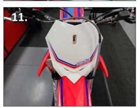
11. Reinstall the rear fender, airbox cover, numberplate/headlight mask, fuel tank assembly, and seat.
