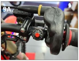
Install the new start (9A) and kill (9B) switches on the handles bars. Once installed plug them into the harness.
