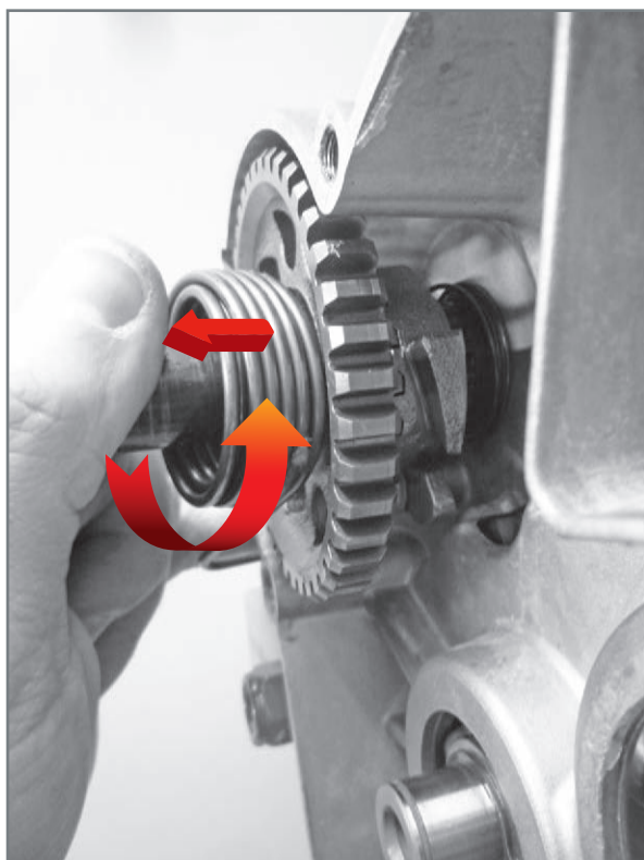
Extraction of shaft from crankcase.
