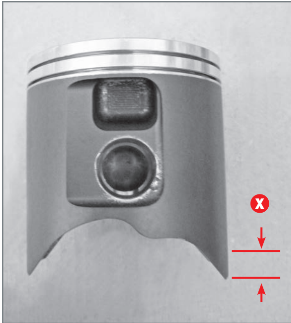
Position to measure the outside diameter of the piston.
