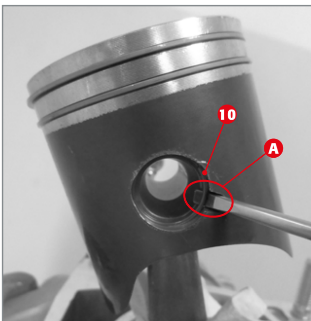
Removal of piston circlip.
