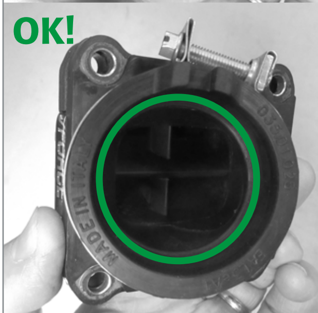
Flow guide positioning.
