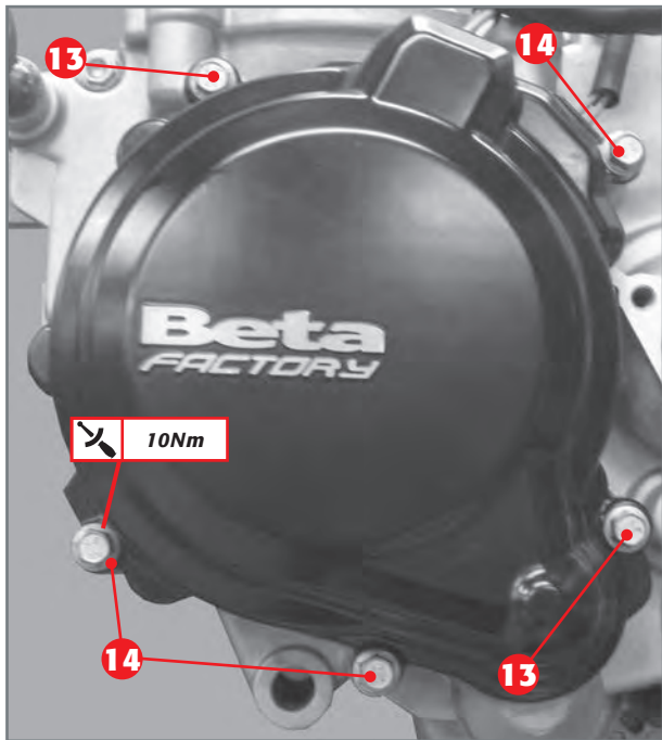
Flywheel cover coupled to crankcase.
