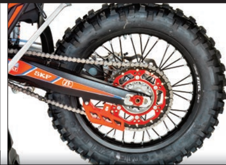
Left: The lithium battery is housed under the seat, which has a push-button to remove the item. It's excellent. Middle: A D.I.D O-ring chain runs on a high-end dual-compound sprocket. The tires are Metzeler 6 Days units that
