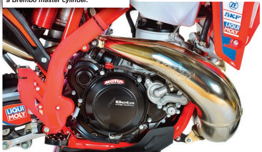
Top: All of the Beta two-strokes are carbureted, the 250RR uses a 36mm Keihin PWK. It comes with special graphics, a seat cover and, of course, the KYB fork. Bottom: The pipe is plated, the clutch is smooth and is managed up top via a Brembo master cylinder.
