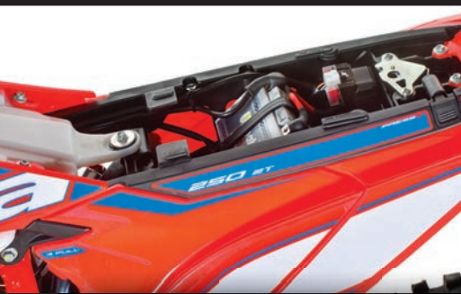
Left: The lithium battery is housed under the seat, which has a push-button to remove the item. It's excellent. Middle: A D.I.D O-ring chain runs on a high-end dual-compound sprocket. The tires are Metzeler 6 Days units that
