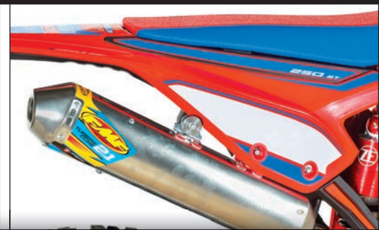
did not get great reviews from our testers. Right: The 250RR comes with a straight-through muffler, but for our needs, a spark arrestor is almost a necessity. The FMF 2.1 Turbine Core is excellent.
