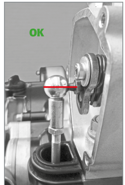
Correct position of the control rod seat.
