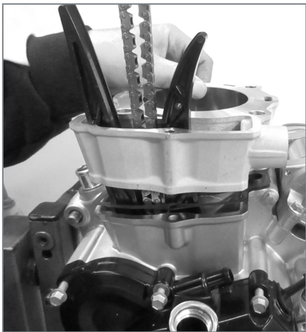
Passing the chain through the cylinder.
