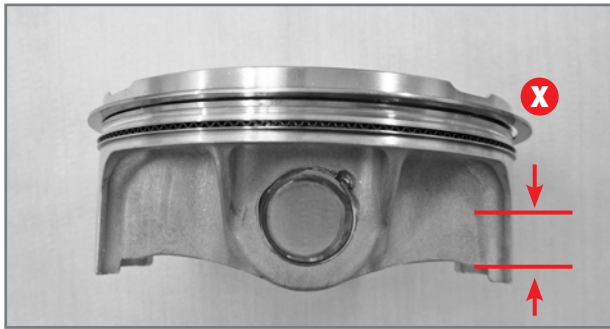
Position to measure the outside diameter of the piston.
