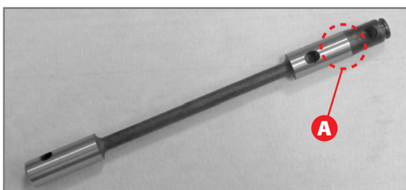
Checking oil pump control shaft.
